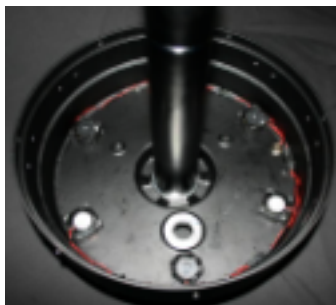
Below – left shows a picture of the primary mirror reinstalled in the rear casting with the locking collar installed. Below – right shows the Feather Touch Microfocuser.
