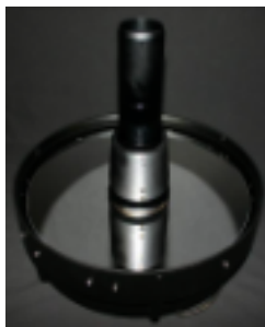
Below – left shows a picture of the primary mirror reinstalled in the rear casting with the locking collar installed. Below – right shows the Feather Touch Microfocuser.
